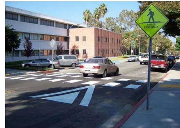
Figure 3.14.2. Typical Raised Crosswalk Application
